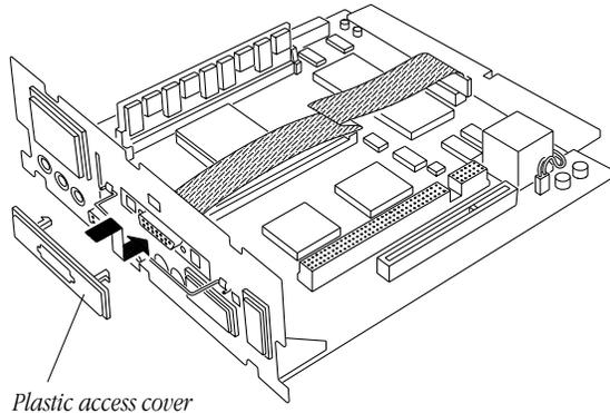
12. Attach the plastic access cover. Check that the video connector protrudes through the opening.
