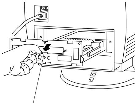
2. Pull down the wire handle on the rear of the logic board. Use the handle to slide the logic board out of the computer.
