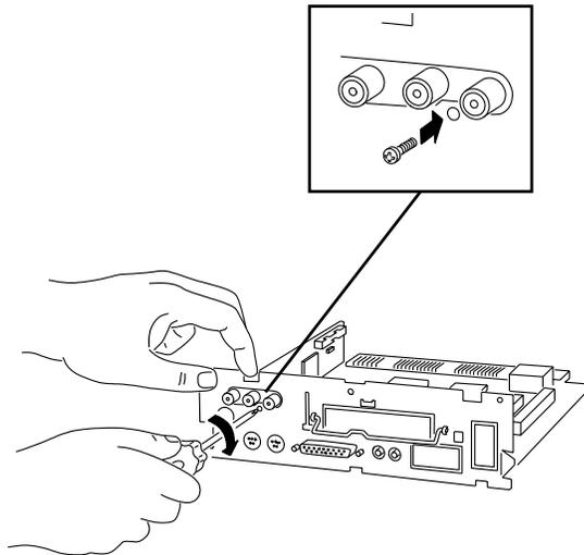
15. Secure the video card to the rear plate using a self-tapping screw. Do not over-tighten.
