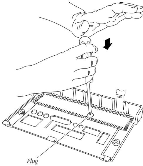
6. Punch out the plug on the rear panel to clear the port access hole for the TV tuner.
