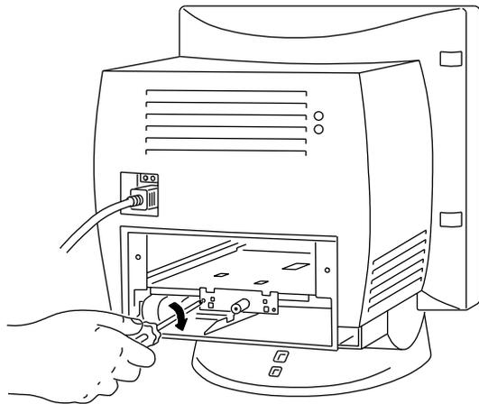
5. Install an attachment screw to secure the TV tuner card.
