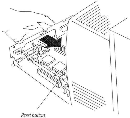
16. Insert the logic board into the channel but do not yet install it all the way.
