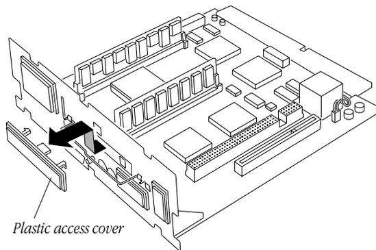
7. Remove the plastic access cover. Compress the tabs and pull it from the metal retainer.
