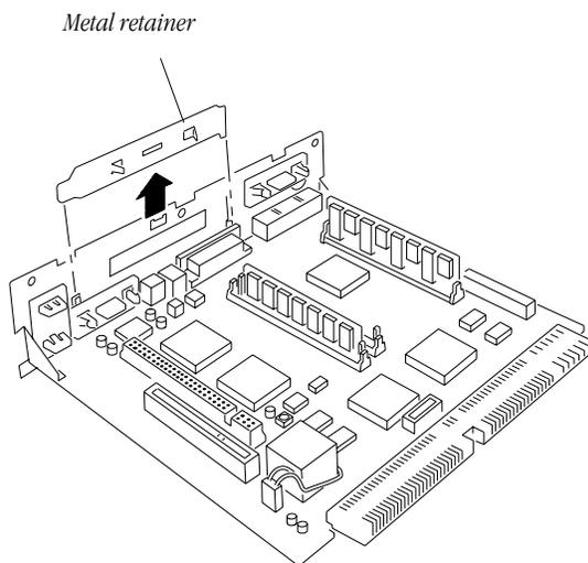
8. Remove the metal retainer.
