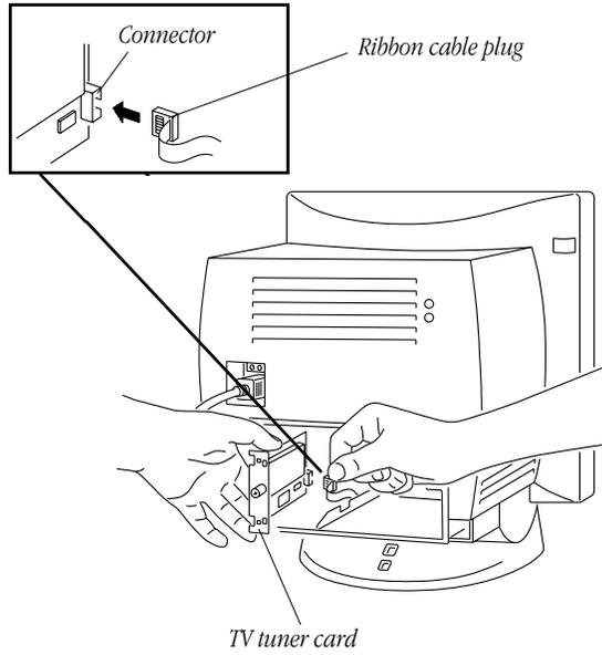
3. Locate the ribbon cable under the logic board tray, and attach it to the connector on the TV tuner card.
