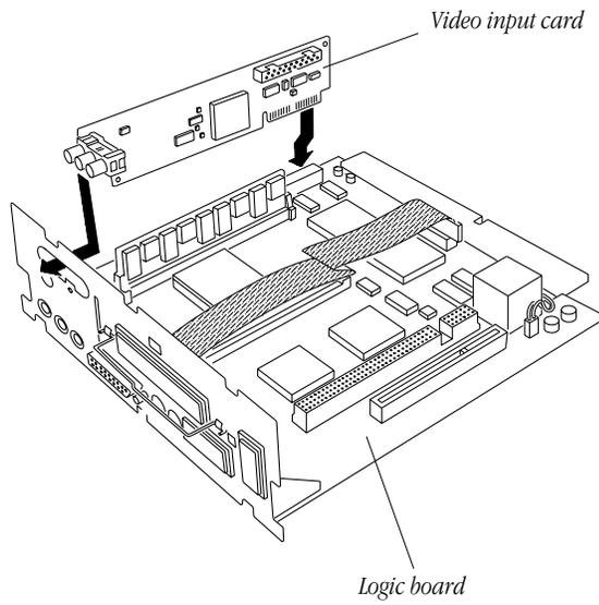
14. Connect the video input card to the logic board.
