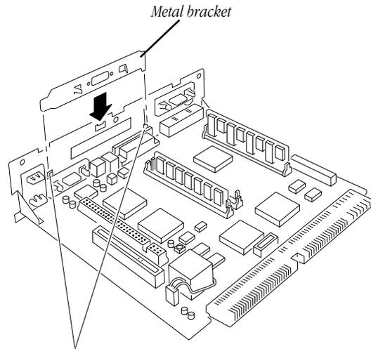
*The metal bracket is correctly seated when it engages these two hooks.*
