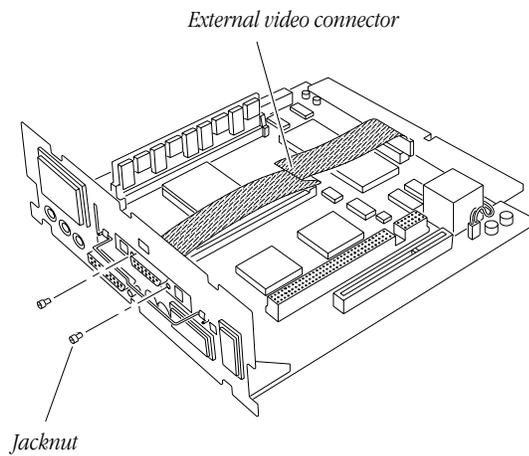
10. Connect the small card on the end of the external video connector to the monitor-out slot on the logic board.
