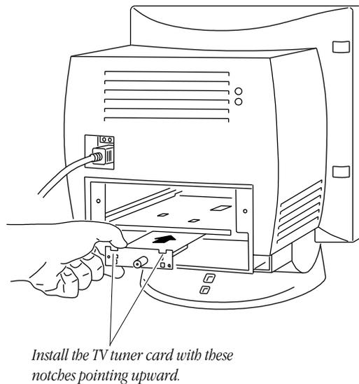
4. Slide the TV tuner card into the channel under the logic board tray. Check that the notches point up.
