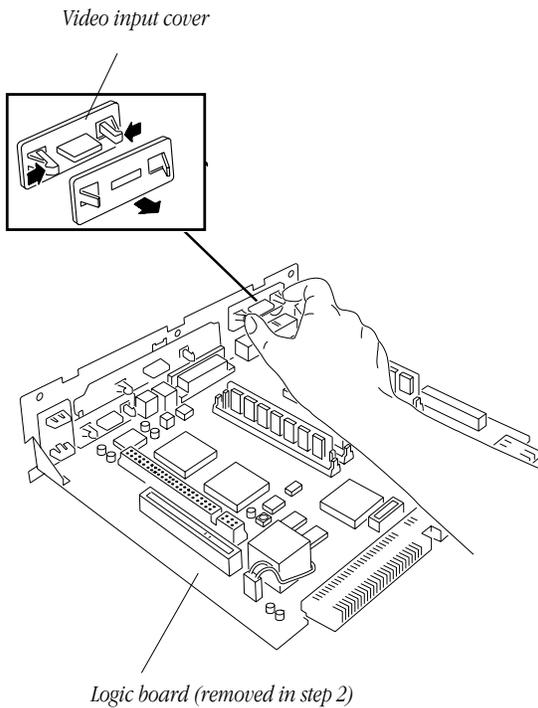
13. Remove the video input cover from the rear plate of the logic board to clear the port access hole.
