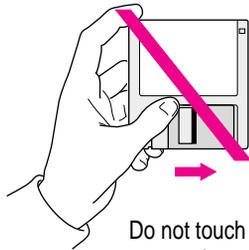
Do not touch the exposed part of the disk behind the metal shutter.
