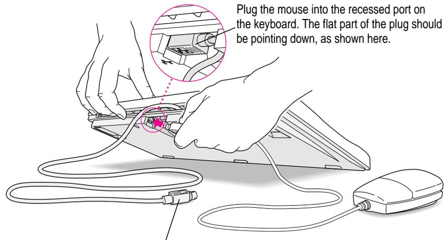
This cable plugs into the Apple Desktop Bus (ADB) port on the back of the computer. The ADB port on the computer is marked with the ⌘ icon.
