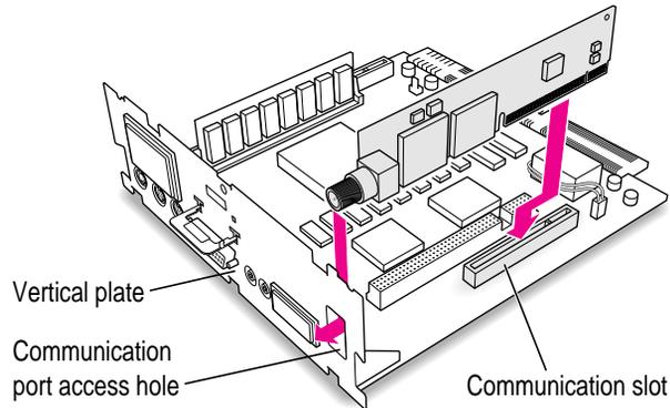
**5** Press down on the card until the connector is solidly in place.
